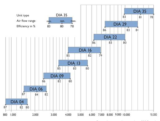
External pressure drop supply air 300 Pa, exhaust air 300 Pa Efficiency of energy recovery acc. to DIN EN 308 (dry condition)
